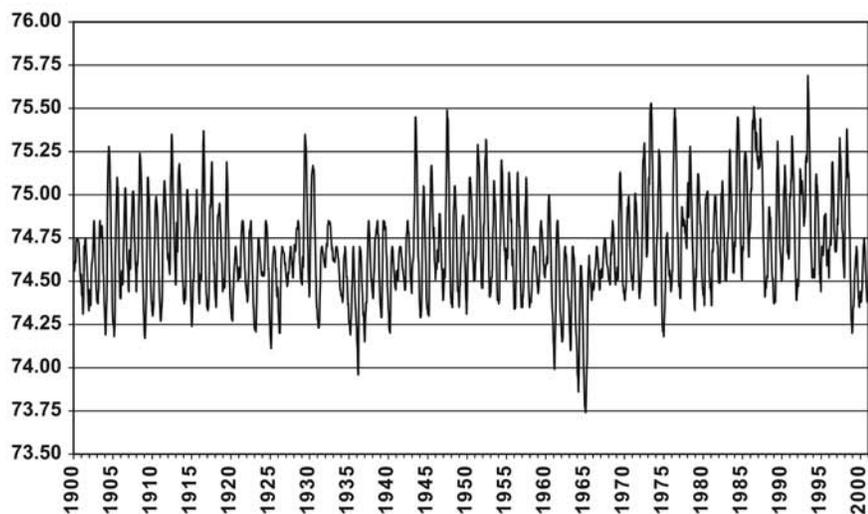
**FIG. 9.** Hydrographs for Lake Ontario showing predicted lake levels if regulation plans 1958DD, X, and Y were implemented using total basin supplies for the period 1900–2000. Plans X and Y were created from 1958DD but allowing more low lake levels to occur during low water-supply periods.
